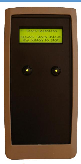
The DPSS® Net is an easy to use tool which allows vessel crew to conduct network storm tests.
